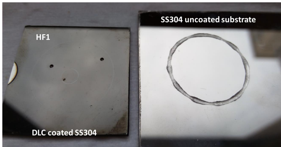
Figure 8: Optical micrograph of the DLC coated (left) and uncoated (right) stainless steel substrates after the pin-on-discs test. The DLC coated sample does not show visible failure, while the bare substrate shows clear evidence of adhesive wear.
