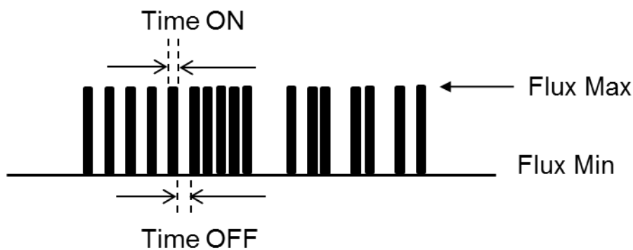
Figure 3. An example of N4E Pulsed Monomer Injector valve operation mode. Monomer flow variant between an open max and a closed minimum flow with fixed time on pulses and variable frequency.
