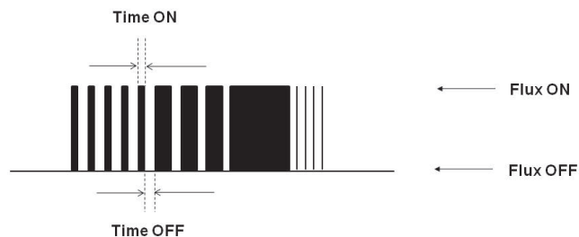
Figure 2: An example of Pulsed Monomer Injector valve operation mode. The total monomer flow variant between an open max and a closed minimum flow with fixed time on pulses and variable frequency.
